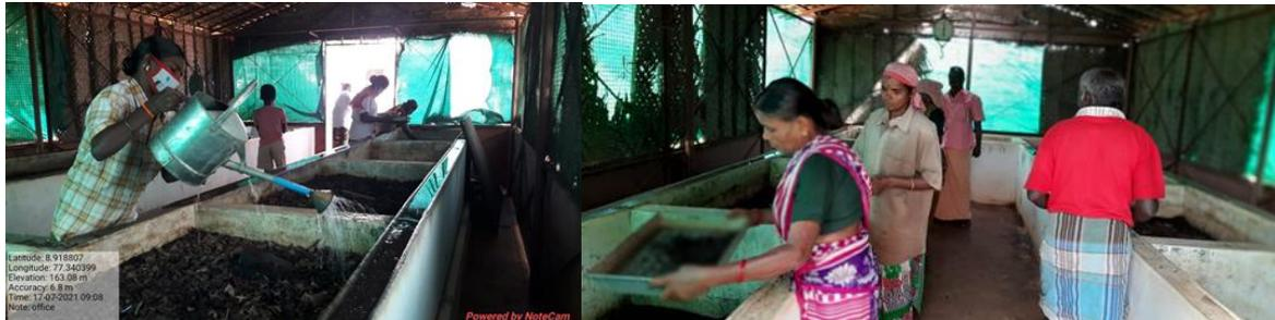
Collection of garbage from all homes and segregation of the same is carried out by the Thooimai Kavalars. At the SWM yard, biodegradable is shredded before being laid on the vermi bed for further processing and generation into vermi compost.
