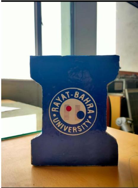
According to the team members the tiles are antistatic, antibacterial and antimicrobial, which means, that they are fungus resistant and static charge defusing; capable of bearing load capacity of 3.5 tonnes. Further, they can sustain temperatures up to 110 degrees centigrade and show no deformation in shape or weight when immersed in water for two days. In the event of any damage, the tiles can be reused for manufacture again.
